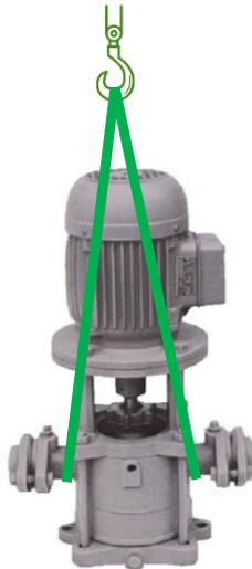
**ATTENTION** The crane device and the ropes must have the appropriate dimensions. The ring eye of the motor must not be used to transport the entire pump unit.
